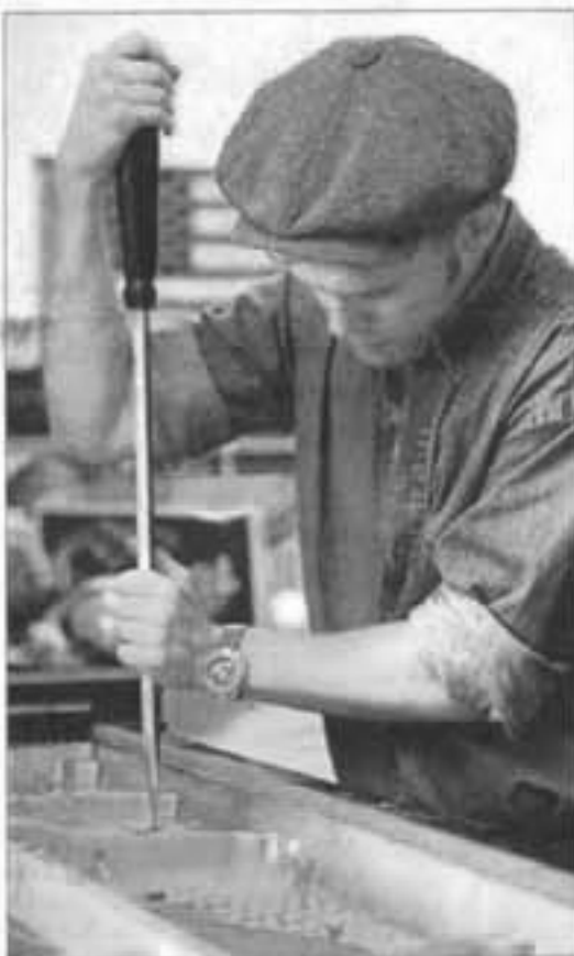
Evan Belschner (above) uses steel wool on Sept. 18 to hand rub the lacquer finish on the lattice-cut front panel from an 1880s Bechstein upright piano being restored at Grand American Piano in Moscow.
