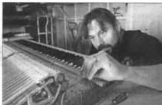
Grand American Piano owner Clint Hughes (above) regulates the action from a 1936 Steirway Model B being restored.
